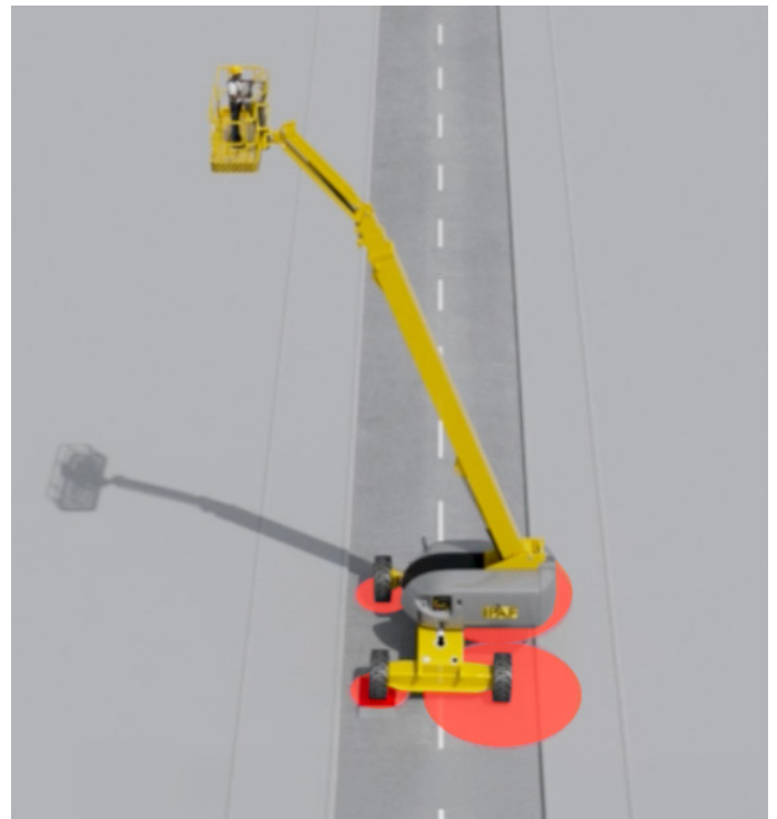
4. When retracted and elevated the highest load is on the two tyres directly under the counterweight
