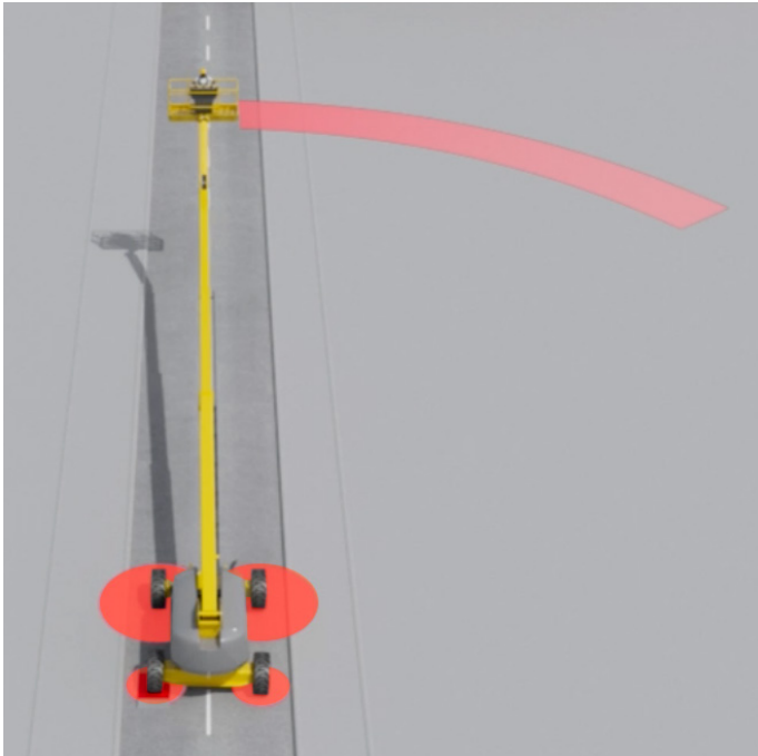
1. When the boom is near horizontal the highest load is on the tyres nearest the platform
