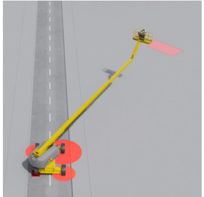
2. As the boom rotates in the horizontal position the highest load is on the tyre nearest the platform
