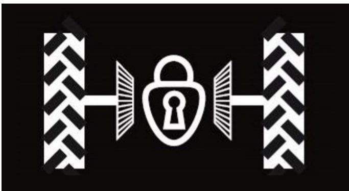
Differential lock decal example (credit Niftylift)
