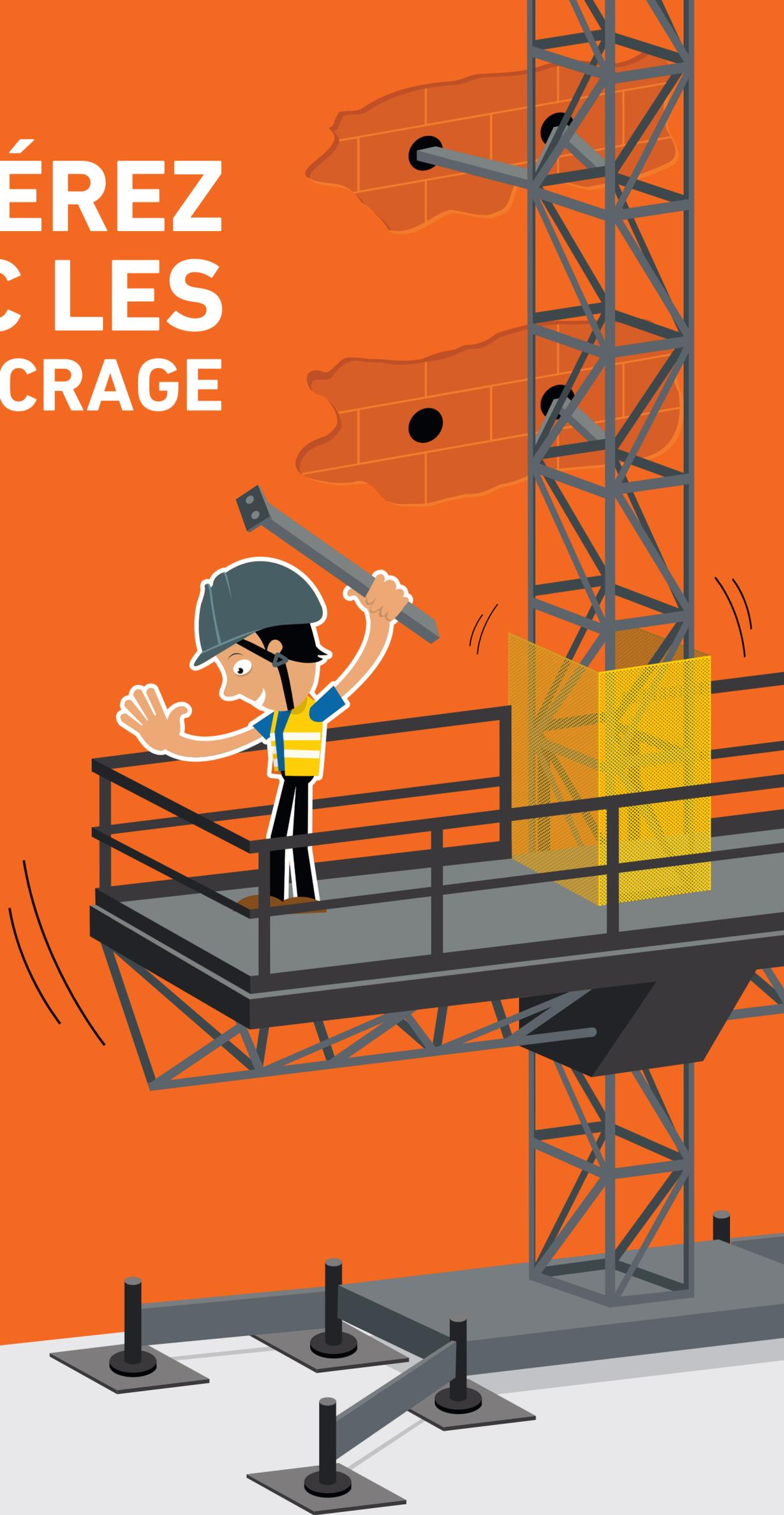
**LA PLATEFORME DE TRAVAIL SUR MÂT A BESOIN DE TOUS SES POINTS D'ANCRAGE POUR ÊTRE STABLE**
