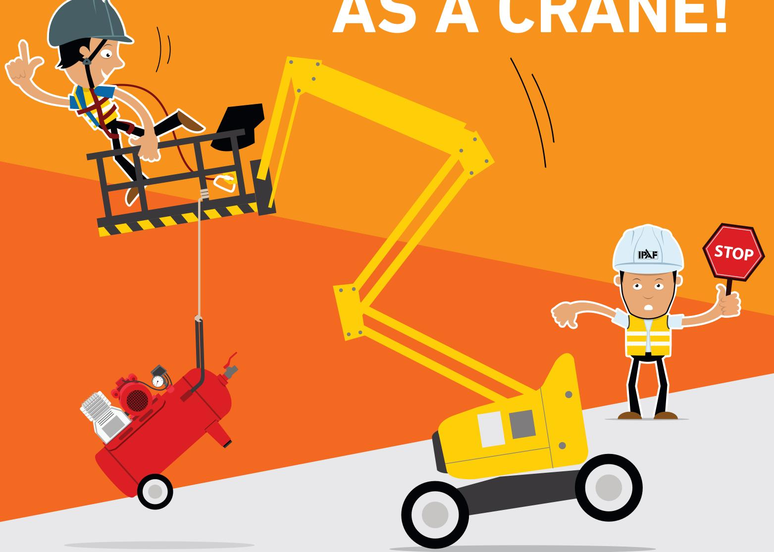
LIFTING OBJECTS CAN OVERLOAD OR DAMAGE THE MEWP AND CAUSE IT TO OVERTURN
