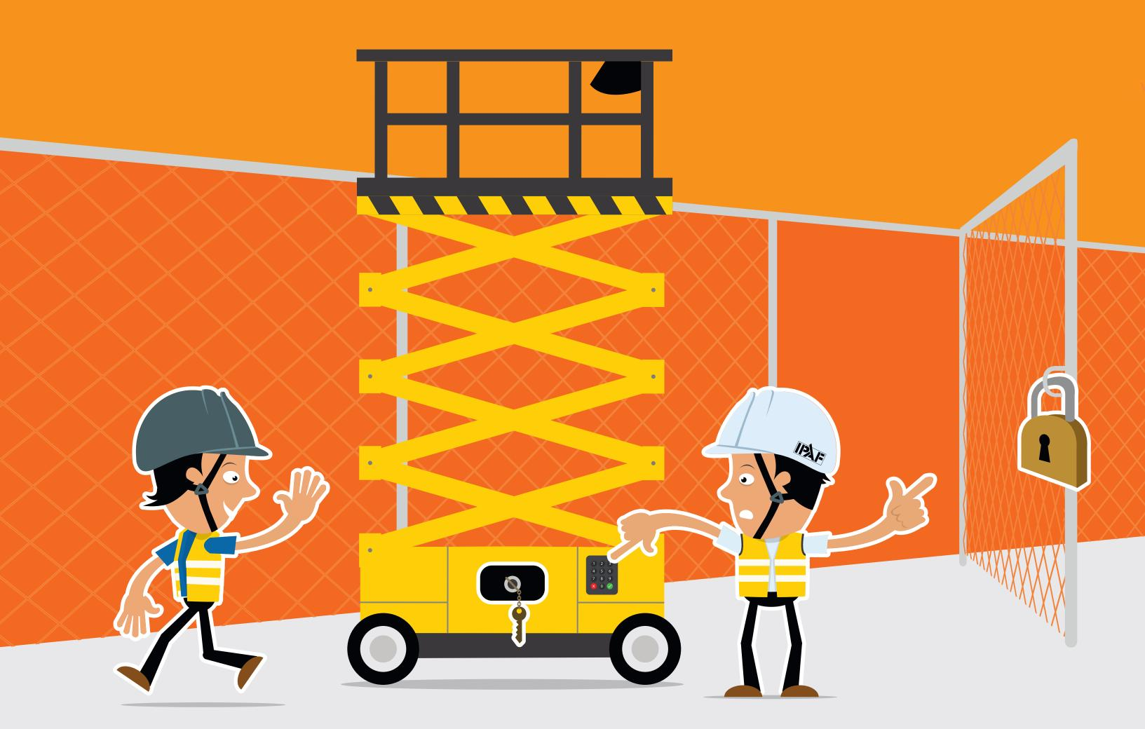
AFTER USE, ALWAYS LEAVE THE MEWP IN A SAFE AND SECURE PLACE AND REMOVE THE KEY
