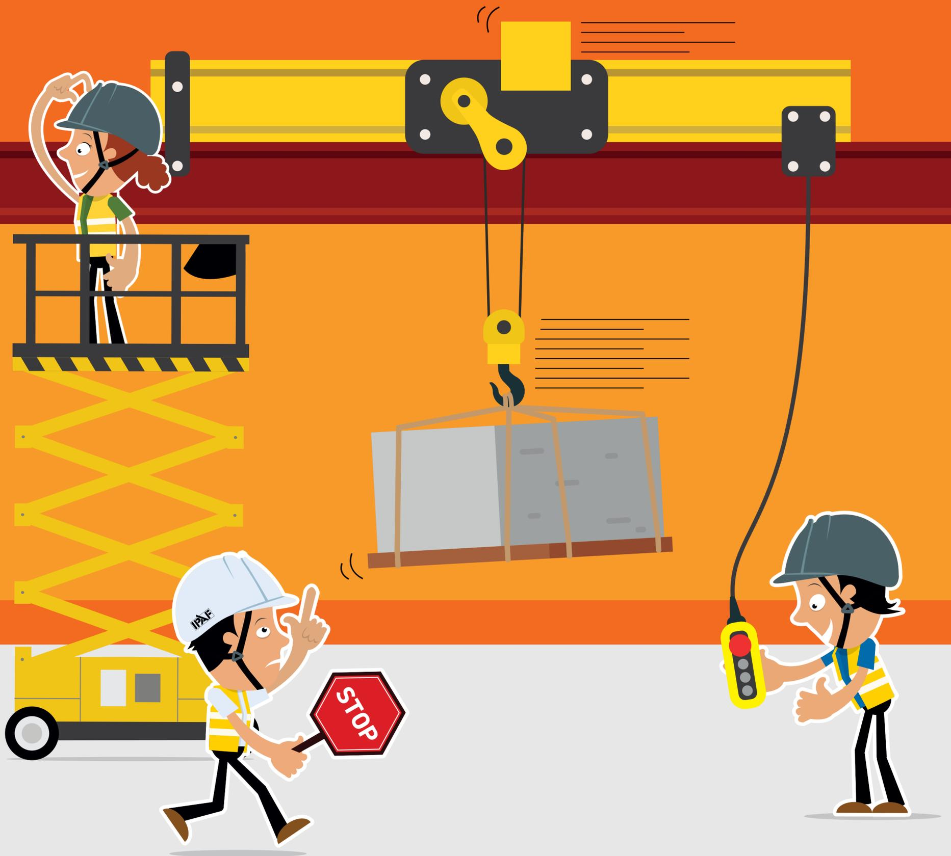
**NE JAMAIS ÉLEVER LA PLATE-FORME S'IL Y A UN RISQUE D'ÊTRE PERCUTÉ PAR D'AUTRES ÉQUIPEMENTS**
